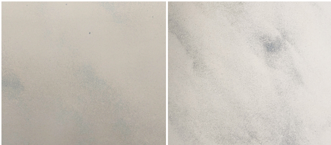
Cast Finish Mediablast Finish Figure 3.3 Organic Dispersion
