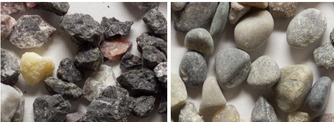
Crushed Stone (Preferred) Rounded Stone Figure 3.2 Aggregate Geometry
