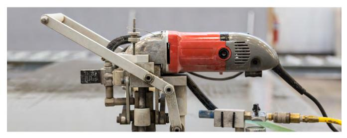
Installers for projects with concealed anchors should be prepared to drill panels in the field. The KEIL Portable Drilling Machine is REQUIRED for drilling concealed anchor attachment holes. Drilling machines can be purchased or rented through TAKTL. Please contact your TAKTL Project Manager for more information and review the following instructions thoroughly before operating the machine.
