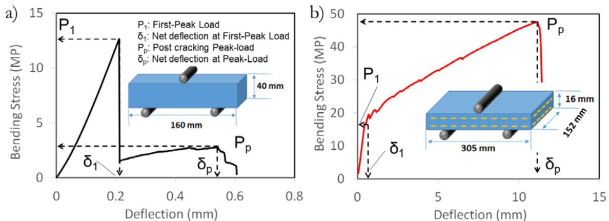
**Figure 3** Typical bending stress-deflection curves for, a) 40x40x160 mm UHPC prisms (2.0 vol.% inorganic fibers) and b) 305x152x16 mm composite UHPC cladding panels with 2D mesh reinforcements and 1.5 vol.% or inorganic fibers.
