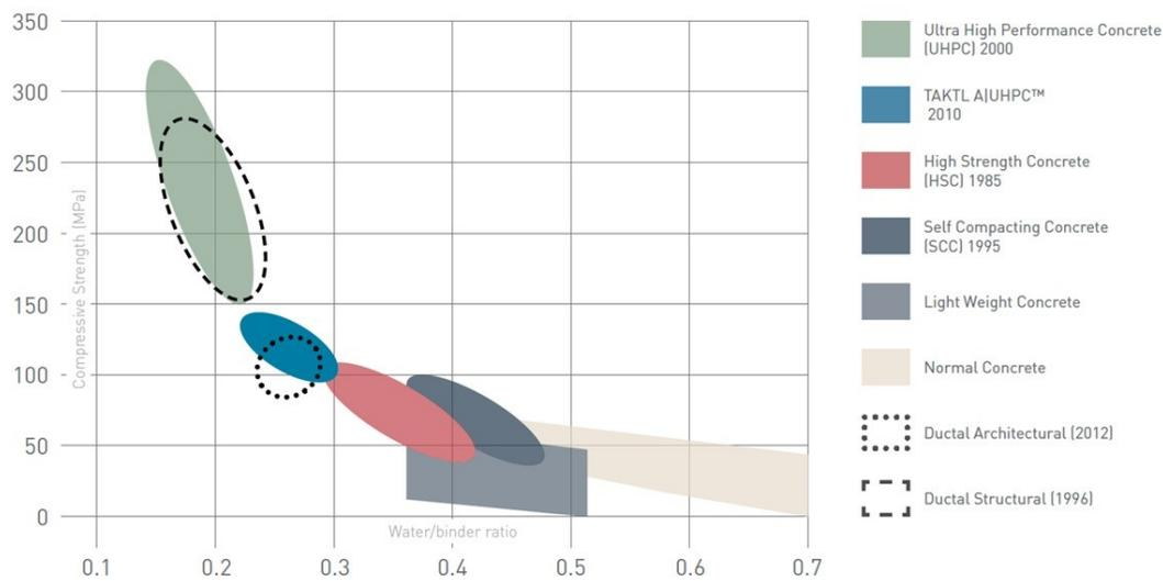
**Figure 2** Classification of concrete according to compressive strength and water to binder ratio (based on CSBT report, 2005; fib, 2009; Batoz et al., 2011; Rigaud et al., 2012; Envel, 2016; Eklips, 2017; Cladia, 2017; Ductal®, 2017).
